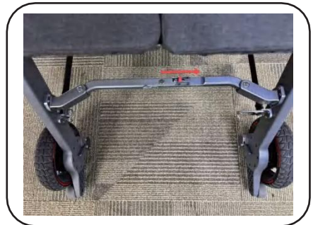
2. Release the Rod Lock at the back of the Roamate.
