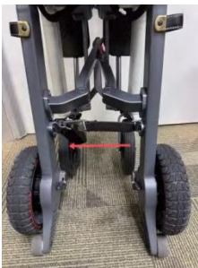
7. Fasten the elastic strap under the battery compartment to secure the seat.
